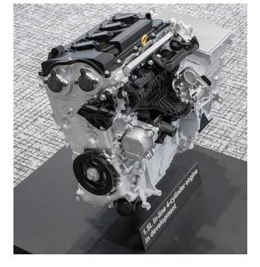
New 1.5L engine Optimized for the electrification era "Electric-Rich" HEVs/PHEVs that capture greater efficiency with electric power unit
