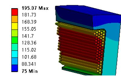
End windings immersed in thermallyconductive potting material
