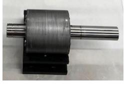
Electrical machine components have been fabricated, including stator with winding and RTDs, housing, and two permanent magnet rotors
