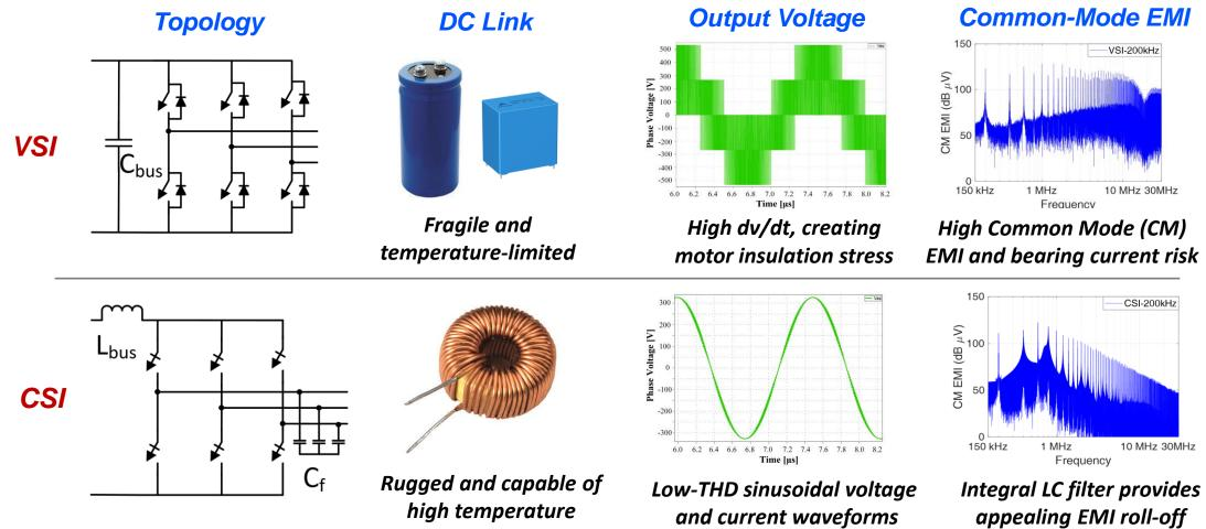
WBG-based Current-Source Inverter (CSI) overcomes many of the VSI limitations by significantly lowering output dv/dt stress, CM EMI emissions, bearing current risks, and temperature limitations
