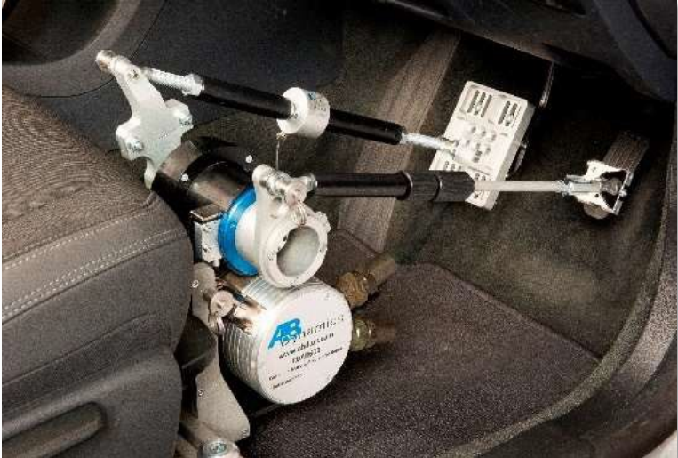
CBAR600 – COMBINED BRAKE AND ACCELERATOR ROBOT
