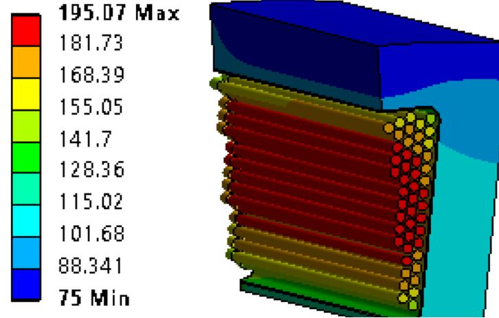
*End windings immersed in thermally-conductive potting material*
