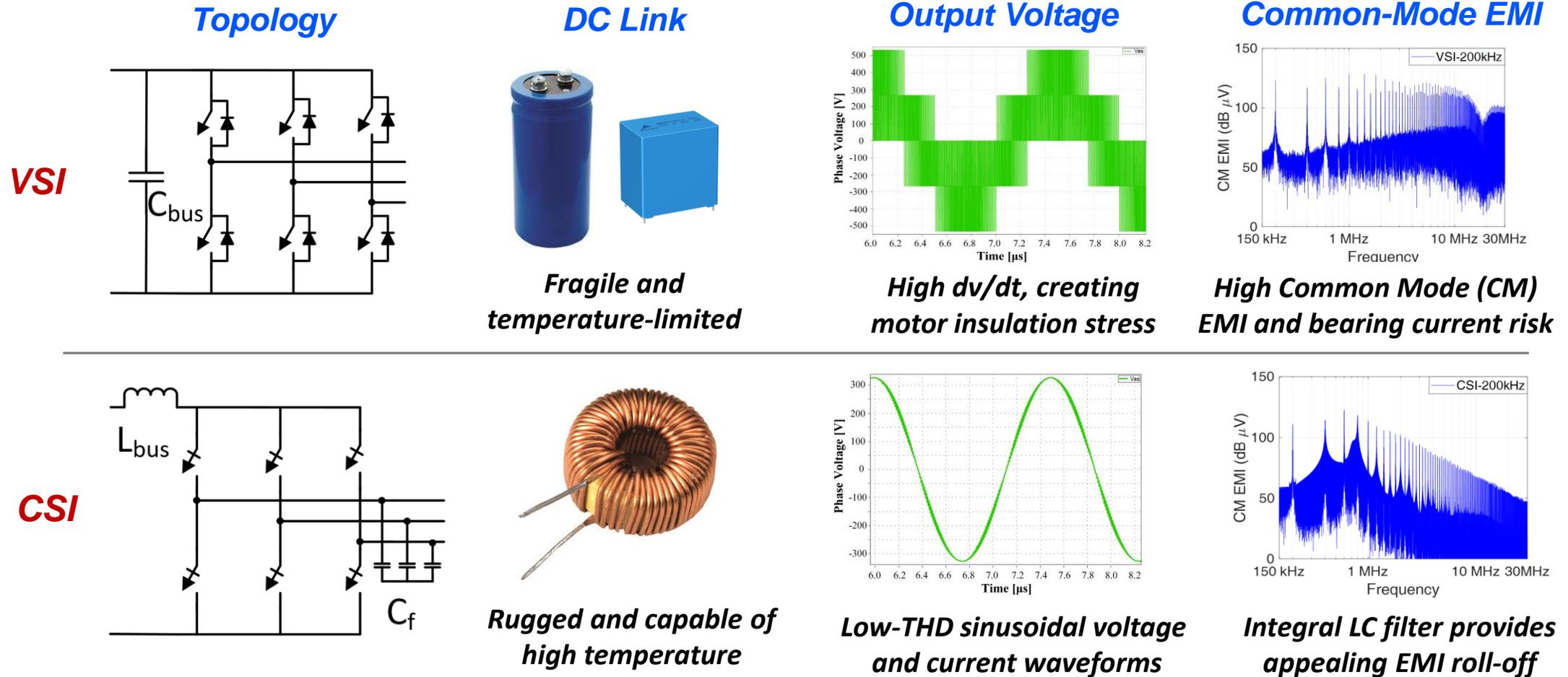
**WBG-based Current-Source Inverter (CSI) overcomes many of the VSI limitations by significantly lowering output dv/dt stress, CM EMI emissions, bearing current risks, and temperature limitations**
