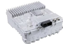
Gen-2 SiC Inverter 43 kW/L, 1050 VDC 115°C Coolant 2020 TRL5/6 440 \mu F DC bus cap Six-Pack SiC modules
