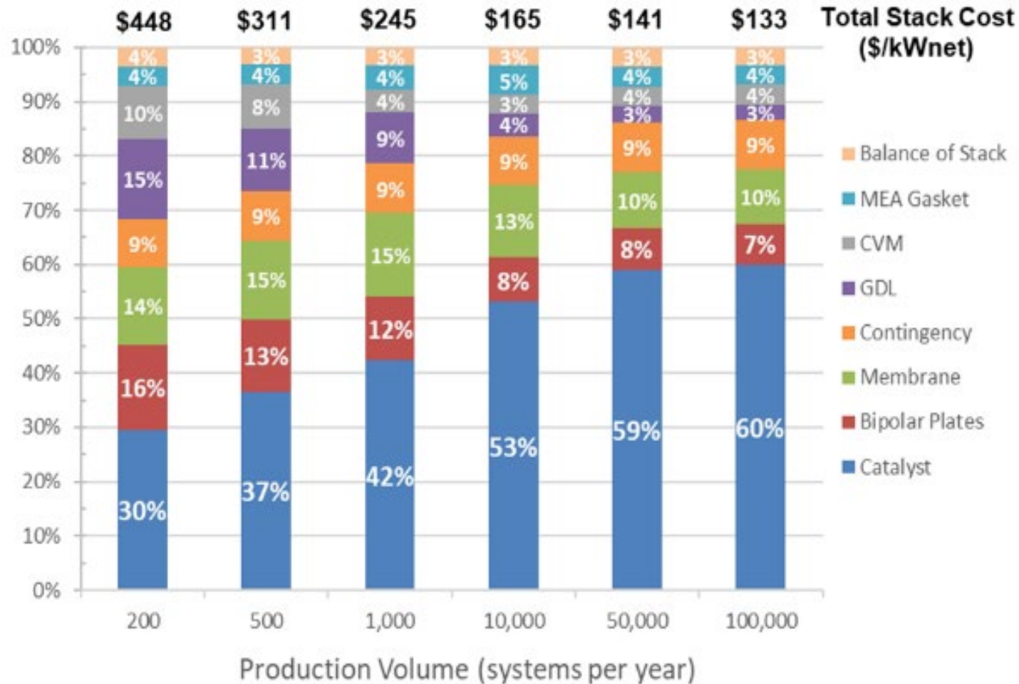
Heavy-Duty Fuel Cell Stack cost breakdown at all production volumes
