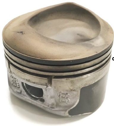
Dense GdZr coating, after 150 hours of operation
