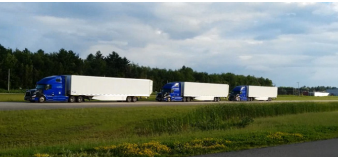
Multiple Test Scenarios: Variation in speed, separation distance, traffic cut-in, etc.
